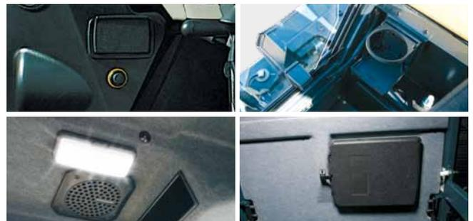
Standard equipment also includes: several handrails, numerous storage spaces, an automatic ceiling light, a bottle holder, 2 x 12V external sockets, one cigarette lighter, one ashtray, a coat rack, a lockable document box...
