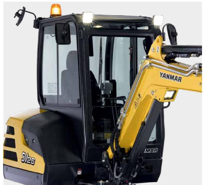
A beacon and 3 additional LED lamps can optionally be added on the cab.
